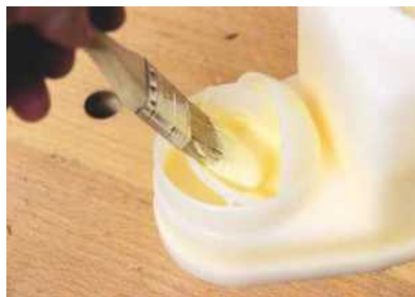
▲ In its normal position, any excess glue can be wiped off on the lip
